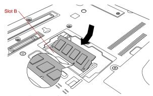
Figure 3-16 Seating the memory module
